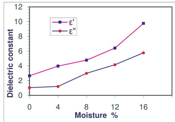
Fig.2-Variation of Dielectric constant and Dielectric loss with moisture content for Clay Loam Soil
