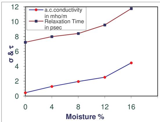
Fig.3-Variation of conductivity and Relaxation time with moisture for Silty clay Soil
