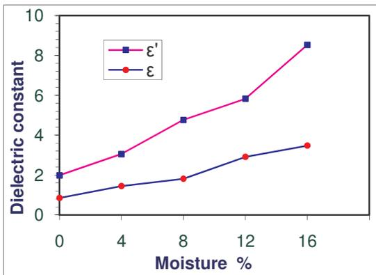
Fig.1-Variation of Dielectric constant and Dielectric loss with moisture content for Silty clay Soil
