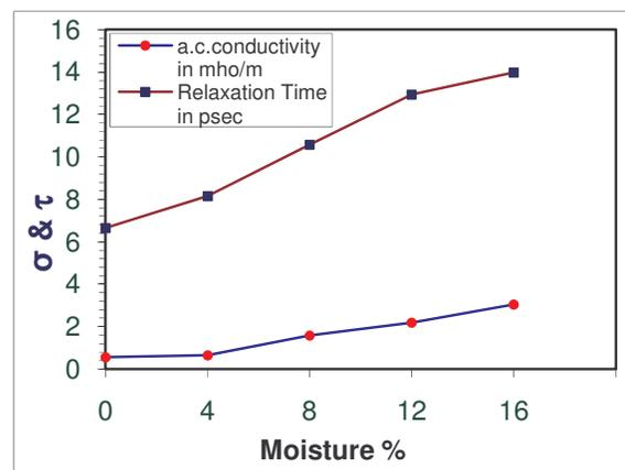
Fig.4-Variation of conductivity and Relaxation time with moisture content for Clay Loam Soil
